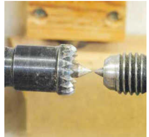
STEP 25. The chucking point is best removed between centres. As I have swivelled the head of the lathe for the hollowing, I need to make sure they are now perfectly aligned
